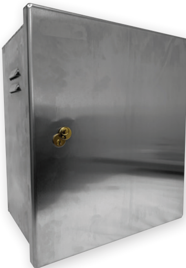
Sturdy .125" 5052 aluminum-sheet cabinet with a Number 2 APL lock.
